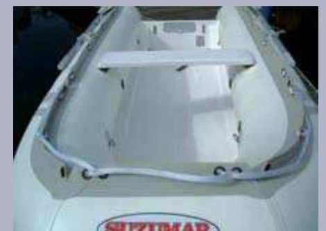
Formed thwart seat and heavy duty transom plate
